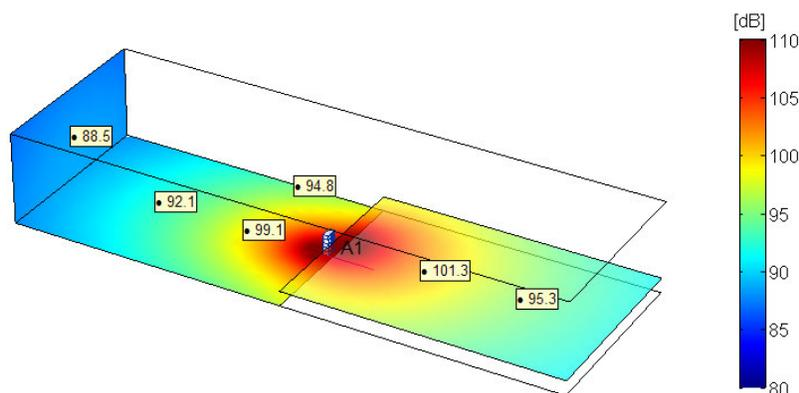
Figure 8: Predicted SPL distribution at 63 Hz (1/3-octave) for the 'standard' bass array using the PSM-BEM models of the cabinets.
