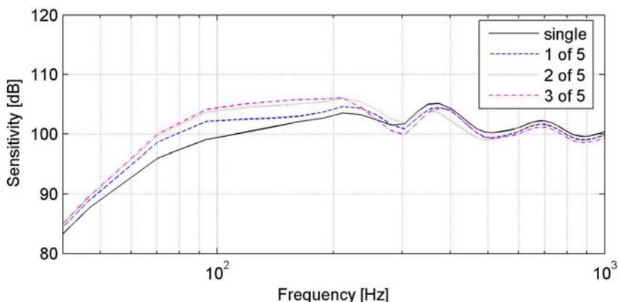
Figure 5: BEM-modelled sensitivity of an unfiltered single bass cabinet compared with the sensitivity of one active cabinet in an array of five (for different positions of the active one in the array).
