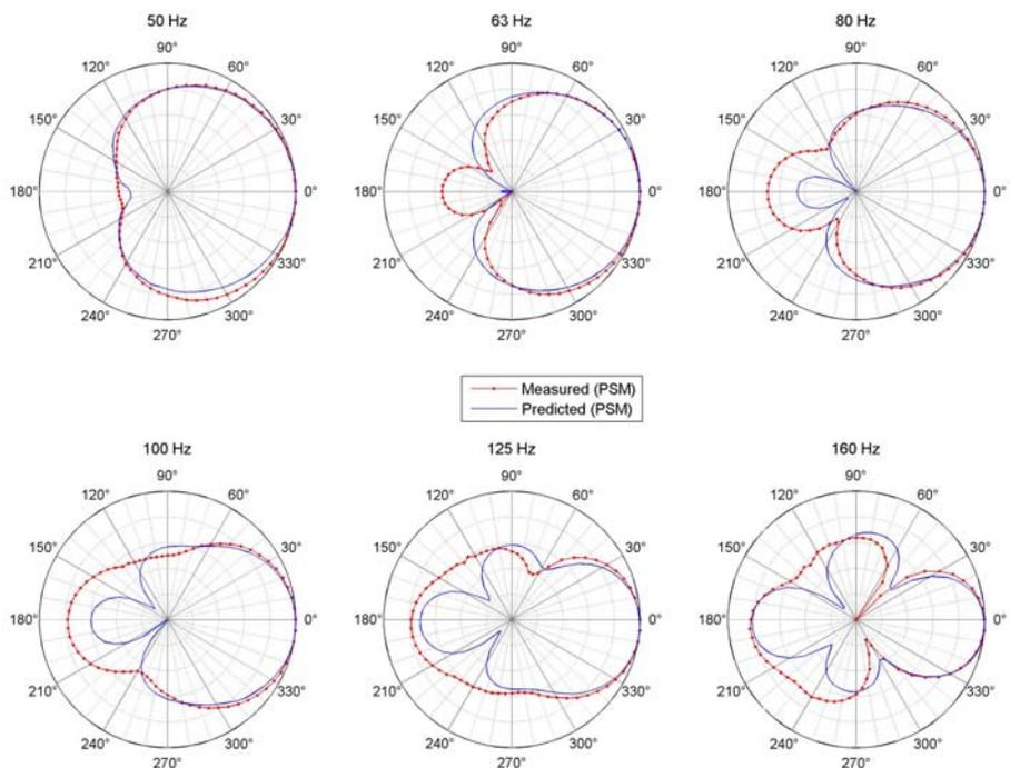
Figure 13: Measured and predicted vertical polar diagrams for the 'cardioid' bass array set-up using the PSM at different 1/3-octave band centre frequencies (6 dB/div).
