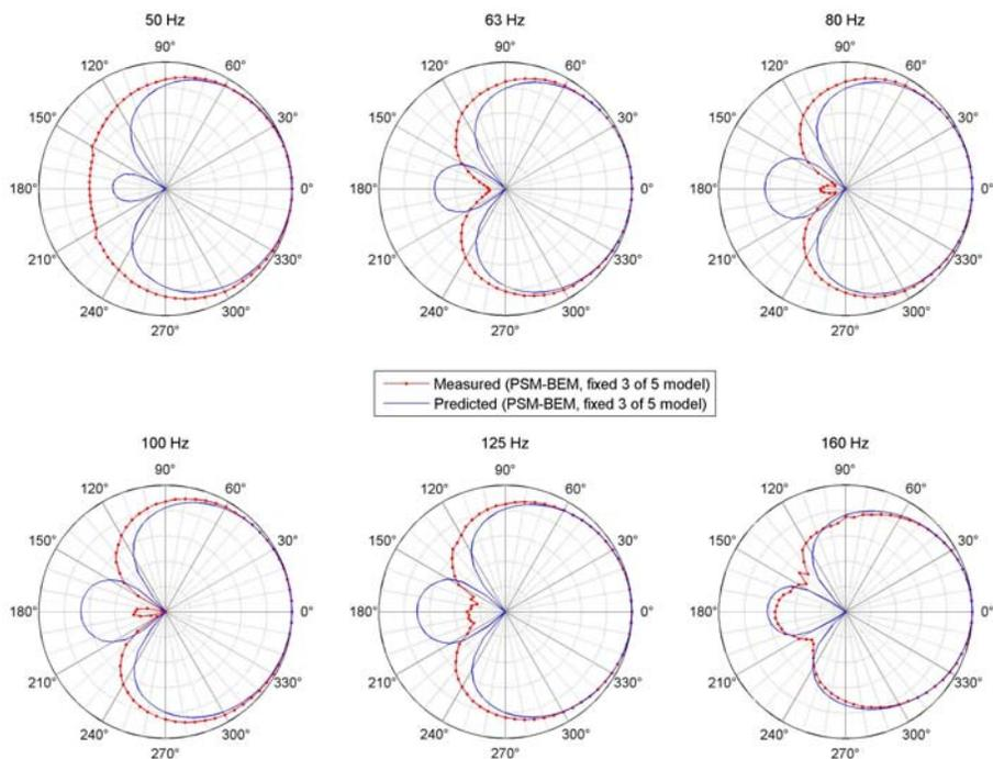
Figure 16: Measured and predicted horizontal polar diagrams for the 'cardioid' bass array set-up using the fixed '3 of 5' PSM-BEM model at different 1/3-octave band centre frequencies (6 dB/div).
