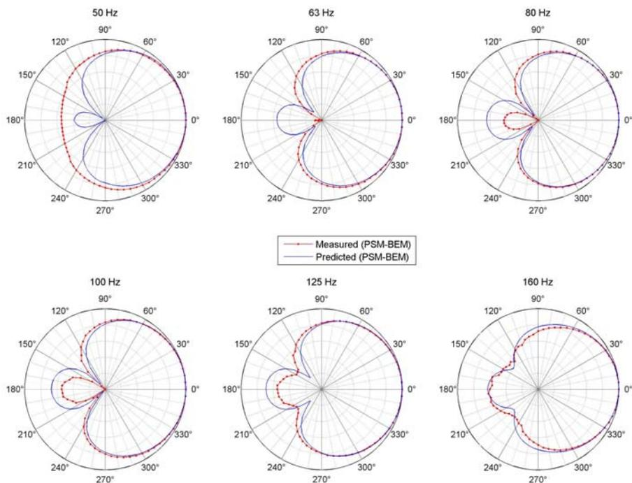
Figure 14: Measured and predicted horizontal polar diagrams for the 'cardioid' bass array set-up using the PSM-BEM model at different 1/3-octave band centre frequencies (6 dB/div).
