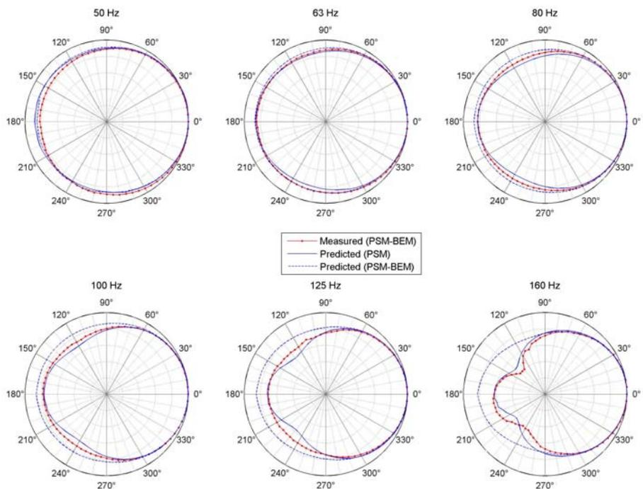
Figure 10: Measured and predicted horizontal polar diagrams for the 'standard' bass array set-up at different 1/3-octave band centre frequencies (6 dB/div).
