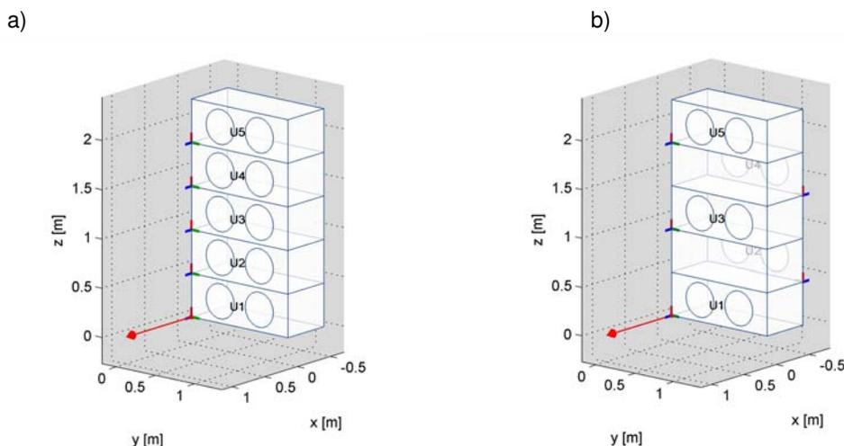
Figure 6: 'Standard' bass array set-up (a) and 'cardioid' bass array set-up (b).
