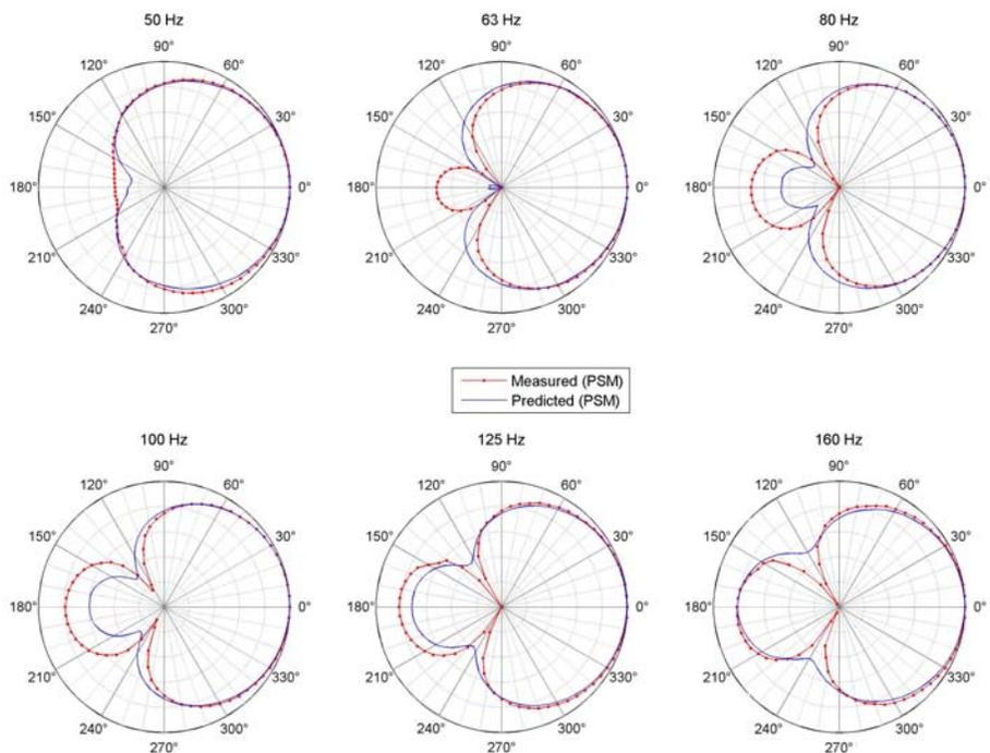
Figure 12: Measured and predicted horizontal polar diagrams for the 'cardioid' bass array set-up using the PSM at different 1/3-octave band centre frequencies (6 dB/div).
