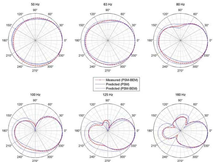
Figure 11: Measured and predicted vertical polar diagrams for the 'standard' bass array set-up at different 1/3-octave band centre frequencies (6 dB/div).
