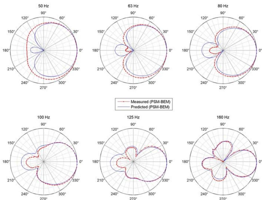
Figure 15: Measured and predicted vertical polar diagrams for the 'cardioid' bass array set-up using the PSM-BEM model at different 1/3-octave band centre frequencies (6 dB/div).
