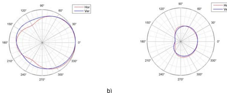
Figure 4: Polar diagram of the magnitude (a) and phase (b) behaviour of one bass cabinet as part of an array of five cabinets at 100 Hz (magnitude diagram: 6 dB/div, phase diagram: 90°/div).
