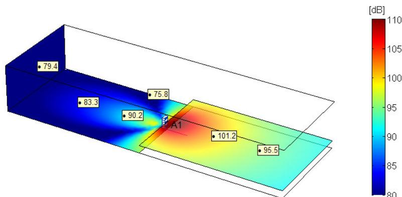
Figure 9: Predicted SPL distribution at 63 Hz (1/3-octave) for the 'cardioid' bass array using the PSM-BEM models of the cabinets.
