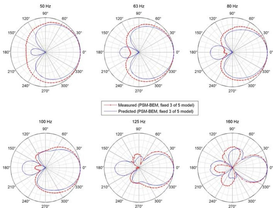
Figure 17: Measured and predicted vertical polar diagrams for the 'cardioid' bass array set-up using the fixed '3 of 5' PSM-BEM model at different 1/3-octave band centre frequencies (6 dB/div).
