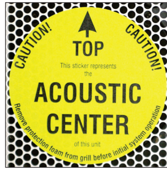
fig.3 Sticker showing acoustic centre and unit orientation
